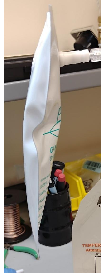
**9. Detach the IsoBag and IsoFlask. Purge the device with air several times before moving on to the next sample.**
