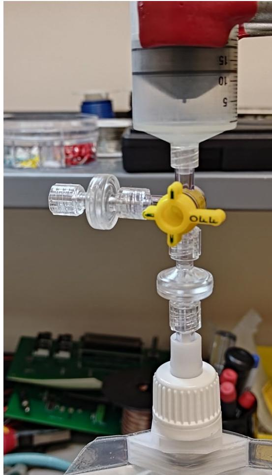
7. Once the device is purged, press the valve of an evacuated IsoBag® into the output (side) port.
