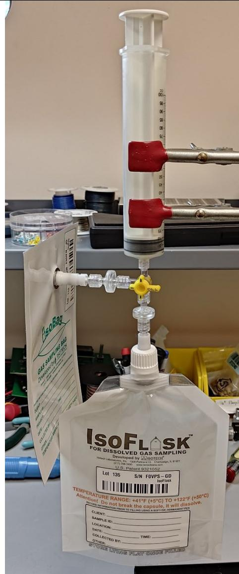
8. Alternately raise and lower the plunger to transfer the gas from the IsoFlask into the IsoBag.
