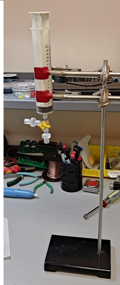
4. Purge the device with air by alternately lifting and lowering the syringe plunger. This will also test the function of the check valves. The gas should inlet through the bottom port, and expel through the side port.
