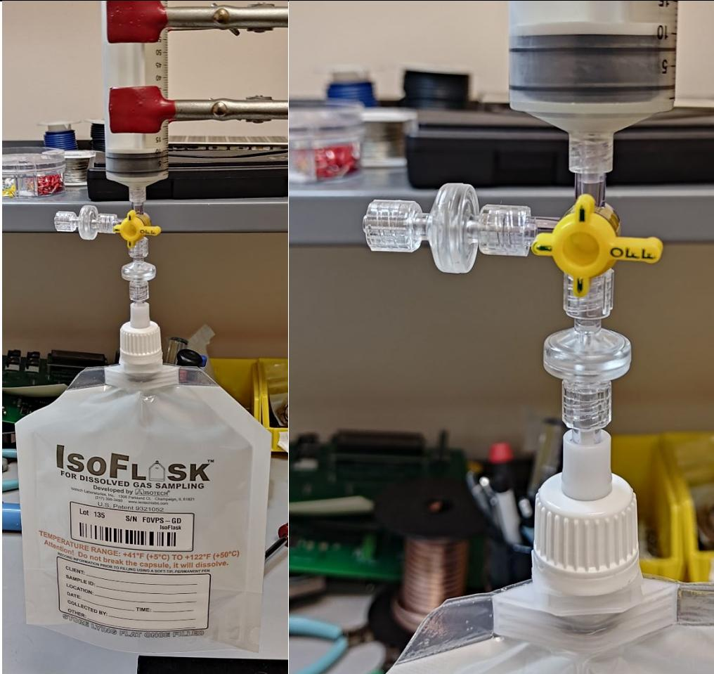
6. Draw up about 10 cc of scrubbed sample and purge through the open side port to remove air from the dead volume. Do this at least twice unless you have extremely limited sample volume.
